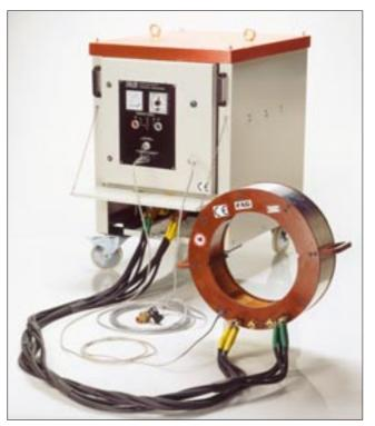
88: FAG low-voltage induction coil with transformer
