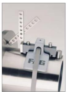
63b: Measuring a tapered roll neck with an FAG Taper Measuring Instrument MGK9205; the stop touches the front datum surface.
