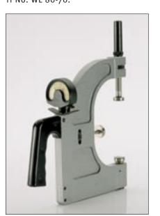
62: Checking the roll neck of a small roll with an FAG dial indicator snap gauge.
