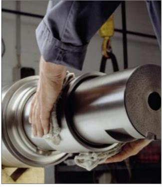
71: Fitting a small cylindrical roller bearing inner ring manually
